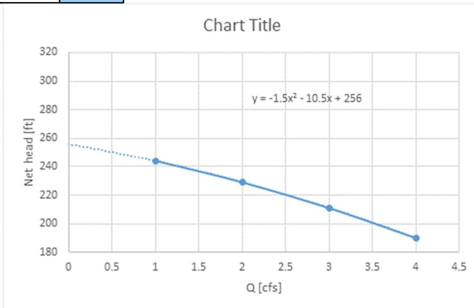
Which suggest a net head of 256 ft at zero flow, rather than something over 310 ft. Could you please provide some guidance as the static head that should be used and the unit designed for? **The friction loss increases as the farmers take more water out of the pressurized line. We are assuming that when the turgo is running at 4 cfs when the farmers are at diverting 100%. That is why the pressure drop is so large due to the friction loss in the pipeline.**
